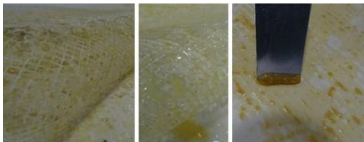
Figure 4. Appearance of the membrane surface and the plastic food-rejection spacer heavily contaminated with biofilm.
